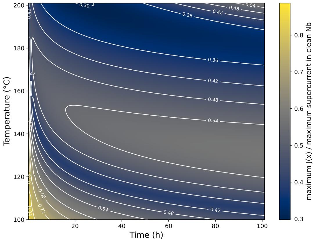
Figure 4.2: Peak Supercurrent Density Variation with Baking Conditions
