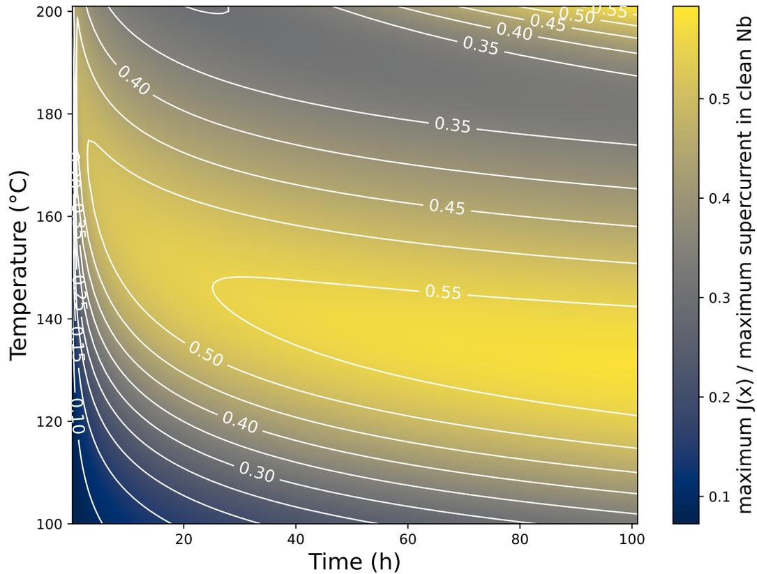
Figure 4.3: Surface Supercurrent Density Variation with Baking Conditions
