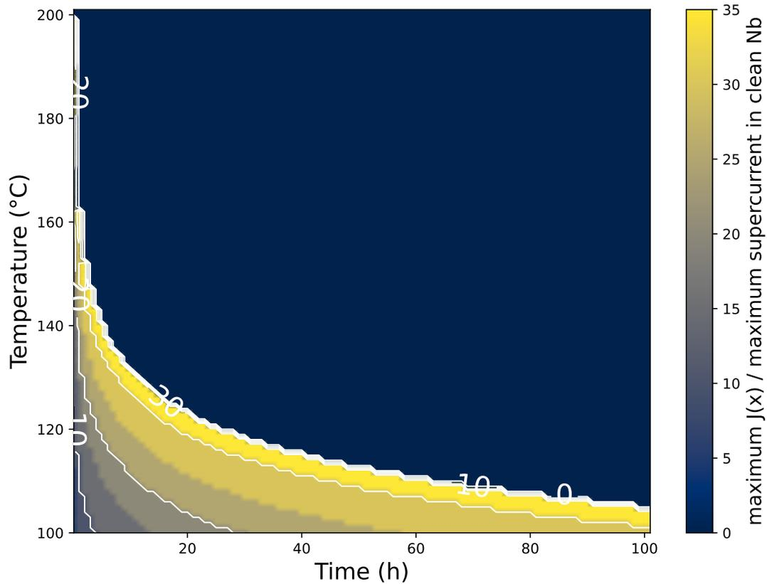
Figure 4.4: Depth of Peak Supercurrent Variation with Baking Conditions
