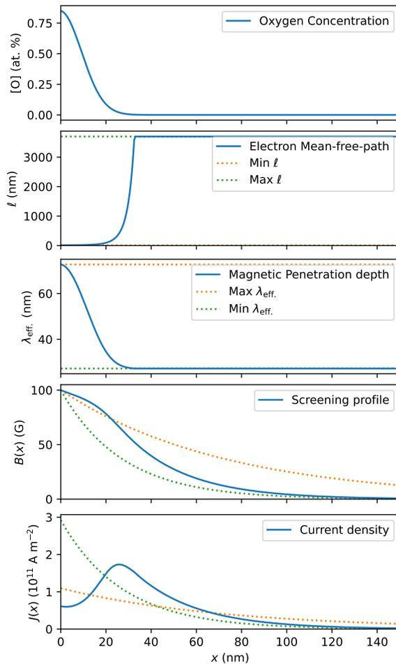
Figure 4.1: Effect on superconducting properties for Baking Conditions: 6 h, 120°C
