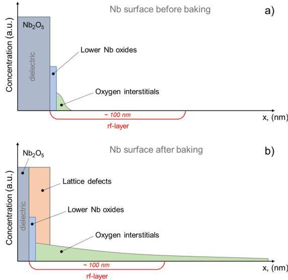
Figure 2.1: Schematic of Surface Layer Oxygen Diffusion Process [25]
